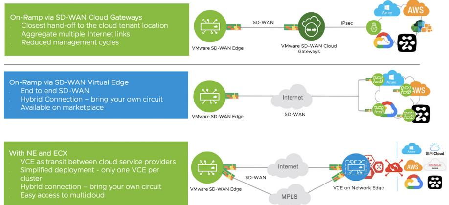
FIGURE 2: VMware SD-WAN enables different connectivity options to the cloud
