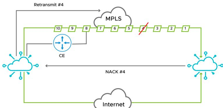
FIGURE 6: Overlay packet retransmission
