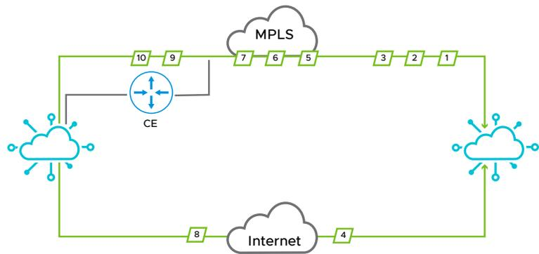
FIGURE 5: Single flow traversing multiple paths across overlay
