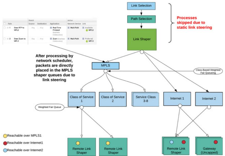
FIGURE 9: Static link steering impact on link scheduler
