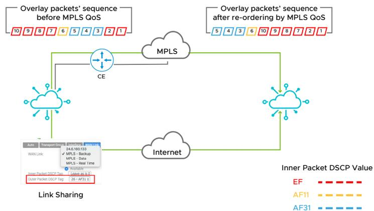
FIGURE 7: Overlay packets being reordered due to MPLS QoS
